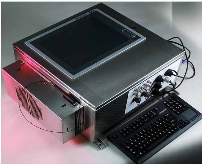
Photo 2: FTA stainless steel NEMA4 box with touch-screen
